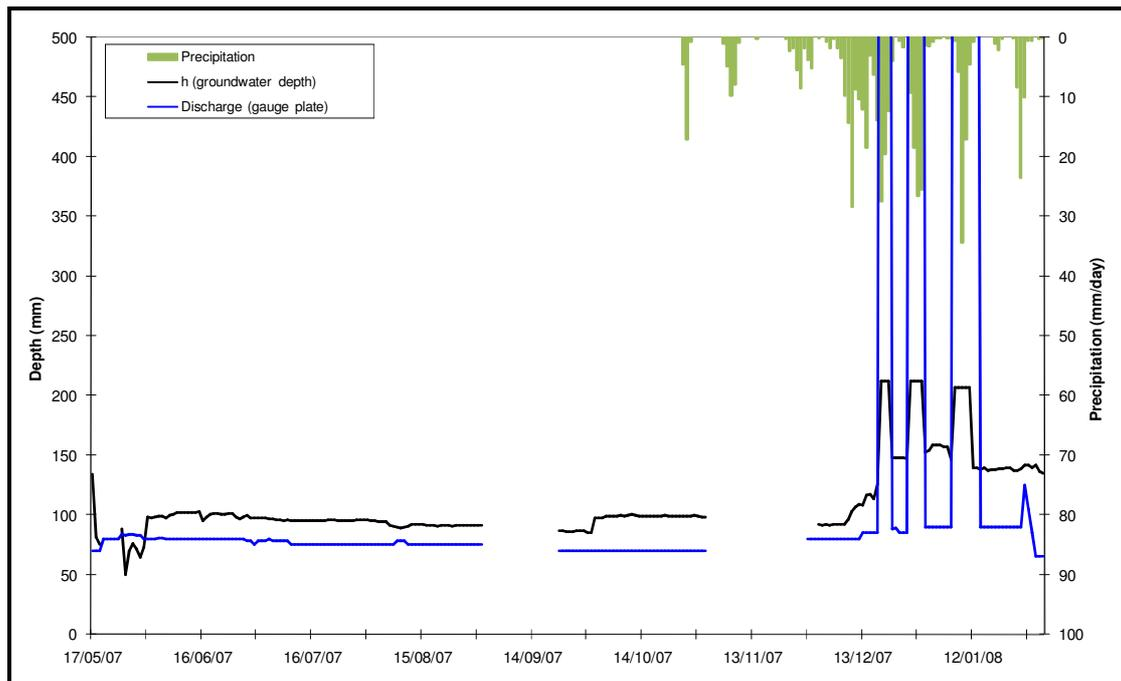
**Figure 4** Variation of groundwater levels with river discharge and precipitation, Mushawe. The results show the availability of groundwater, even during the dry season. Dry season discharge is a result of outflow of groundwater from the top of bridge foundations which function as a sand dam.
