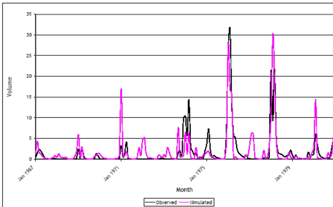
**Figure 3** Observed and simulated runoff, B72E – H catchment, Olifants Catchment.
