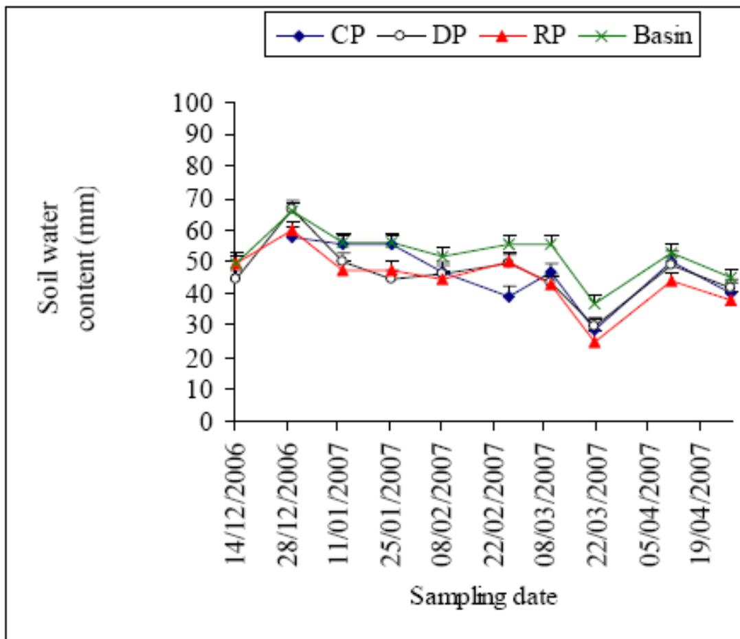
**Figure 6** Soil water content for different tillage practices; CP = conventional ploughing, DP = deep ploughing, RP = ripper.
