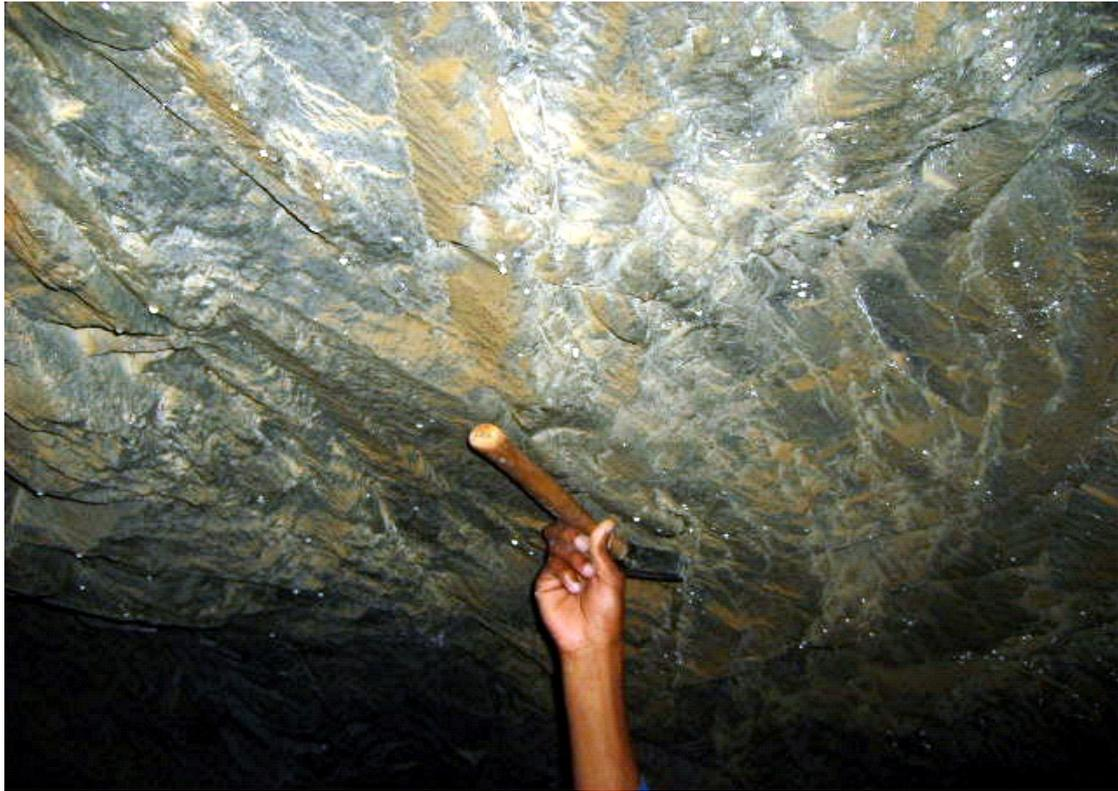
**Figure 5** Measuring fracture orientation for stress analysis, Vubachikwe Mine, Mzingwane Catchment.
