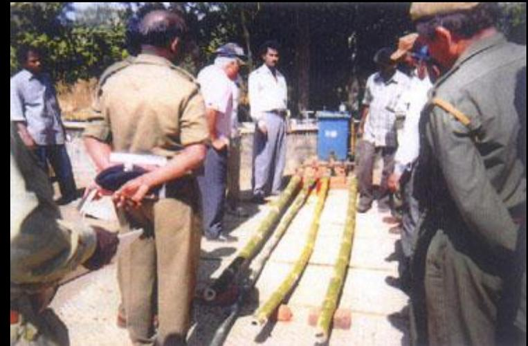
**Photo:** Demonstrating the conventional (or simple) Boucherie technique
